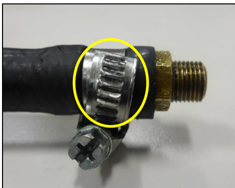
Photo No. 5: Hose clamp/clip in its tightened state, with large portion of threaded band protruding at screw head.
